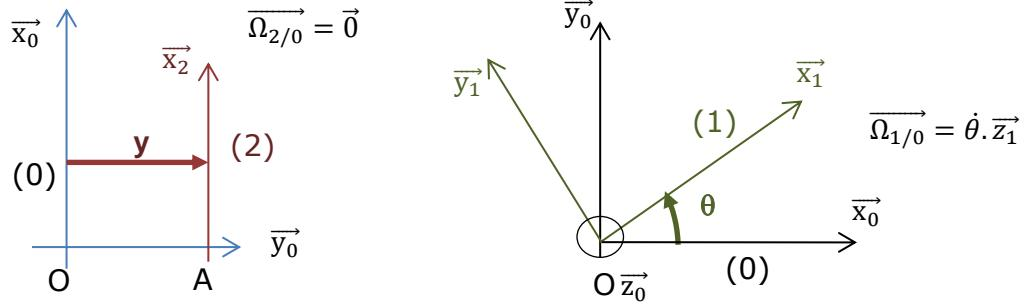
$$\overrightarrow{V_{I,2/1}} = \overrightarrow{V_{I,2/0}} - \overrightarrow{V_{I,1/0}}$$
