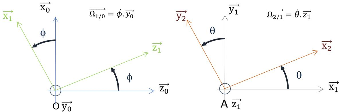
$$\overrightarrow{\Omega}_{3/2} = \vec{0} ; \overrightarrow{\Omega}_{2/0} = \dot{\theta} \cdot \vec{z}_1 + \dot{\phi} \cdot \vec{y}_0 ; \overrightarrow{\Omega}_{3/0} = \dot{\theta} \cdot \vec{z}_1 + \dot{\phi} \cdot \vec{y}_0$$
