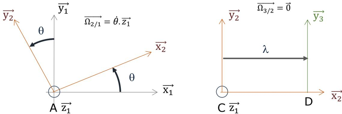
$$\overrightarrow{\Omega}_{3/2} = \vec{0} ; \overrightarrow{\Omega}_{2/0} = \dot{\theta} \cdot \vec{z}_1 ; \overrightarrow{\Omega}_{3/0} = \dot{\theta} \cdot \vec{z}_1$$
