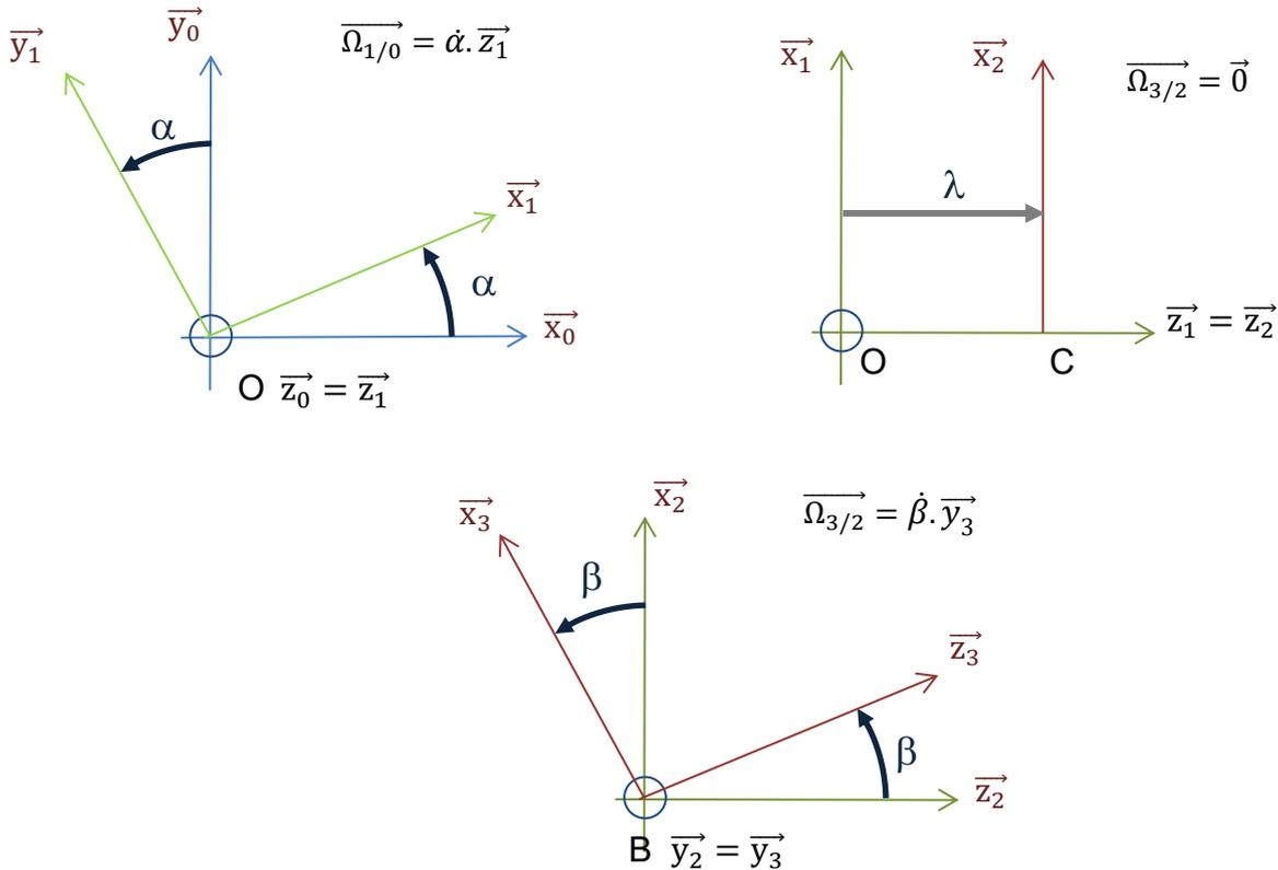
$$\vec{V}_{G \in S3/0} = \frac{d(\vec{OG})}{dt} = \frac{d(\vec{OB} + \vec{BG})}{dt} = \frac{d}{dt} (a \cdot \vec{x}_1 + \lambda \cdot \vec{z}_0 + l \cdot \vec{x}_3)$$
