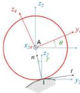
On pose  $O\vec{A} = L\vec{x}_1 + \lambda(t)\vec{z}_0$  et  $I\vec{A} = R\vec{n}$
